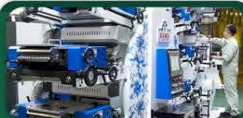
Flexo Letterpress 8 colours + UV + coater + lamination
