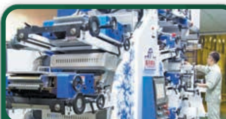
Flexo Letterpress, 8 colours / Corona treater/ Rotary die cutter/ varnish - UV coating/ cold foil/ lamination/ sheeter
